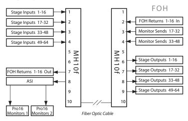
This variation of the 64x48 digital snake example uses two MH10f hubs and fiber optic cabling.
